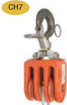
Chance Block - Made of high dielectric, fiberfilled natural nylon - Maximum 1/2" rope - Max Load 3,500 lbs CH7 Double Block Model CH8 Triple Block Model
