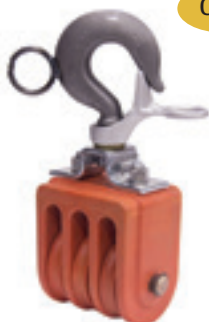
Chance Block - Made of high dielectric, fiberfilled natural nylon - Maximum 1/2" rope - Max Load 3,500 lbs CH7 Double Block Model CH8 Triple Block Model
