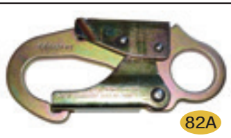
Fixed Eye Double Action Steel Snaphook - Minimum Break Strength 10,116 lbs. - Gate Strength 3600 lbs - Gate Opens .86"
