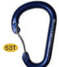
Kong Wire Bent Paddle Carabiner- 22kN Strength 1.25" Opening; 4.5" Length
