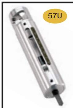
Ripley WS 22A Power Driven End Stripper 3/8" Drill Drive - For 600 volt cables 1/0 AWG to 1000 MCM - Comes with 1 Bushing from chart below
