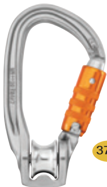
Petzl ROLLCLIP Z TRIACT-LOCK - Min. rope diameter: 7 mm - Max. rope diameter: 13 mm - Max. working load: 2 x 2 = 4 kN - Major axis strength: 20 kN - Minor axis strength: 8 kN - Open gate strength: 7 kN - Approximately 4 1/2"
