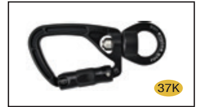
Rock Exotica SwivaEye Carabiner Weight: 5.5oz Breaking Strength: Major Axis: 30 kN; Minor Axis: 7 kN Open Gate: 12 kN; Gate Opening: .84"
