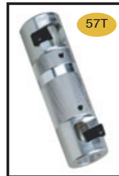
Ripley WS 22 Double-Ended End Stripper - For 600 volt cables 1/0 AWG to 1000 MCM - Comes with 2 Bushings from chart below
