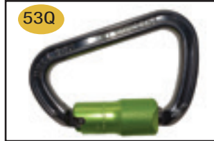
Triple-Action Aluminum Carabiner Min Breaking Strength: 27kN (6,069 lbs) Gate Strength: 16kN (3600 lbs) Opening: .708"
