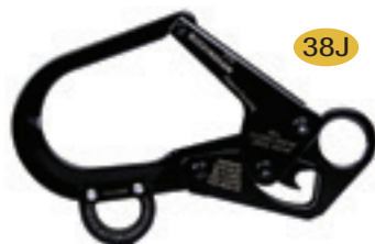
Buckingham Ox hook - WLL of 2,500lbf (gate closed), 1,000lbf (gate open) - 3,600lb. rated locking gate can be locked in the open position
