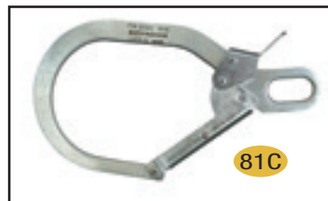
Buckingham Big BuckSnap - Allows the user to easily connect over 4" angle iron. Rounded inner edge designed to prevent damage to conductors when used in hot work applications - 3600lb. rated gate
