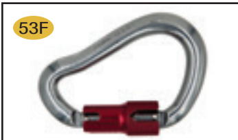
Twist Lock Aluminum Carabiner Min Breaking Strength: 5171 lbs Gate Strength: 3600 lbs Opening: .748"
