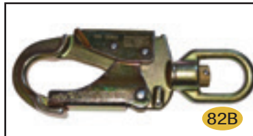
Double Action Forged Steel Swivel Snaphook - Minimum Break Strength 11,240 lbs. - Gate Strength 3600 lbs - Gate Opens .86"
