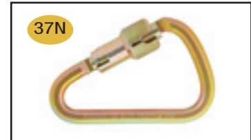
Twist Lock Steel Carabiner Min Breaking Strength: 10,116 lbs Gate Strength: 3600 lbs Opening: 1.06"
